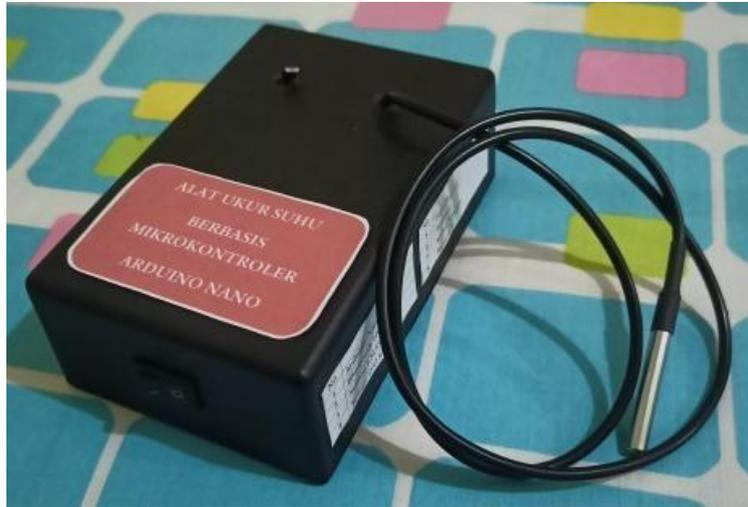
Gambar 2.1 Alat Ukur Suhu Berbasis Mikrontroler Arduino Nano
