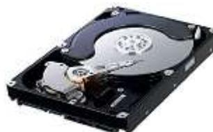
**Gambar 2.5** *Harddisk* (HDD)
